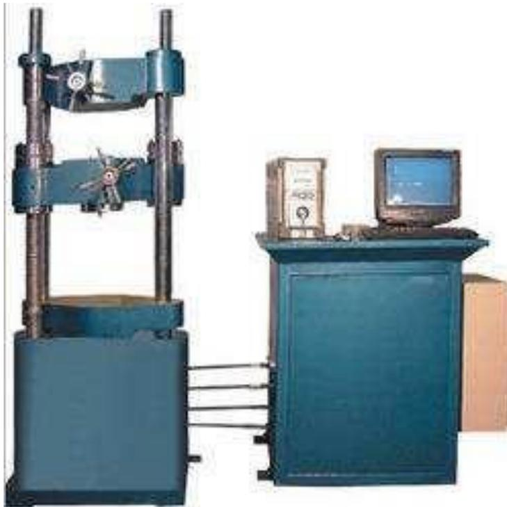
**For ex:** - A specimen of 6 tones capacity gives more accurate result of 10 Tones capacity range instead of 20 Tones capacity range. These ranges of capacity are adjusted on the dial with the help of range selector knob. The control weights of the pendulum are adjusted correctly. The ink should be inserted in pen holder of recording paper around the drum & the testing process is started depending upon the types of test as mentioned below.
